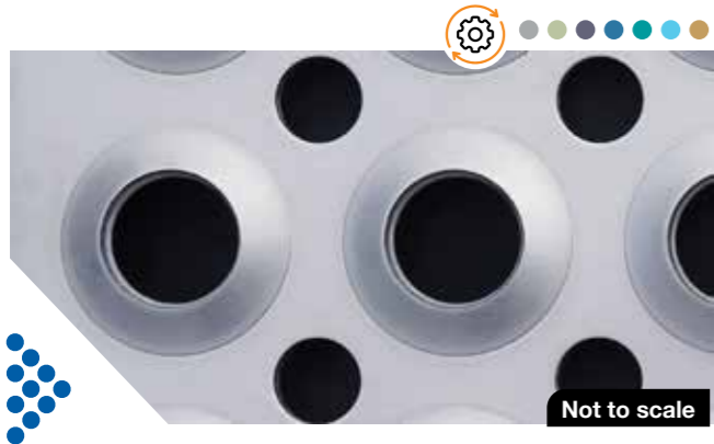
545 | Open area 23% 20.0mm diameter raised holes, 14.0mm diameter drain holes, 45.0mm straight pitch Not to scale
